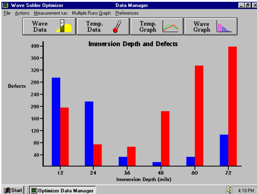
**Figure 4. The second study's immersion depth and defect results**
