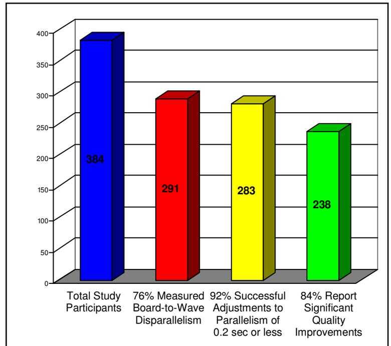
“The Optimizer identified the root cause of chronic skipping defects on our boards. Previous attempts to address this issue resulted in new problems, namely solder shorts. After several Optimizer runs, adjustments were made to eliminate the disparallelism it measured. These modifications had an immediate and positive effect on board quality.”
